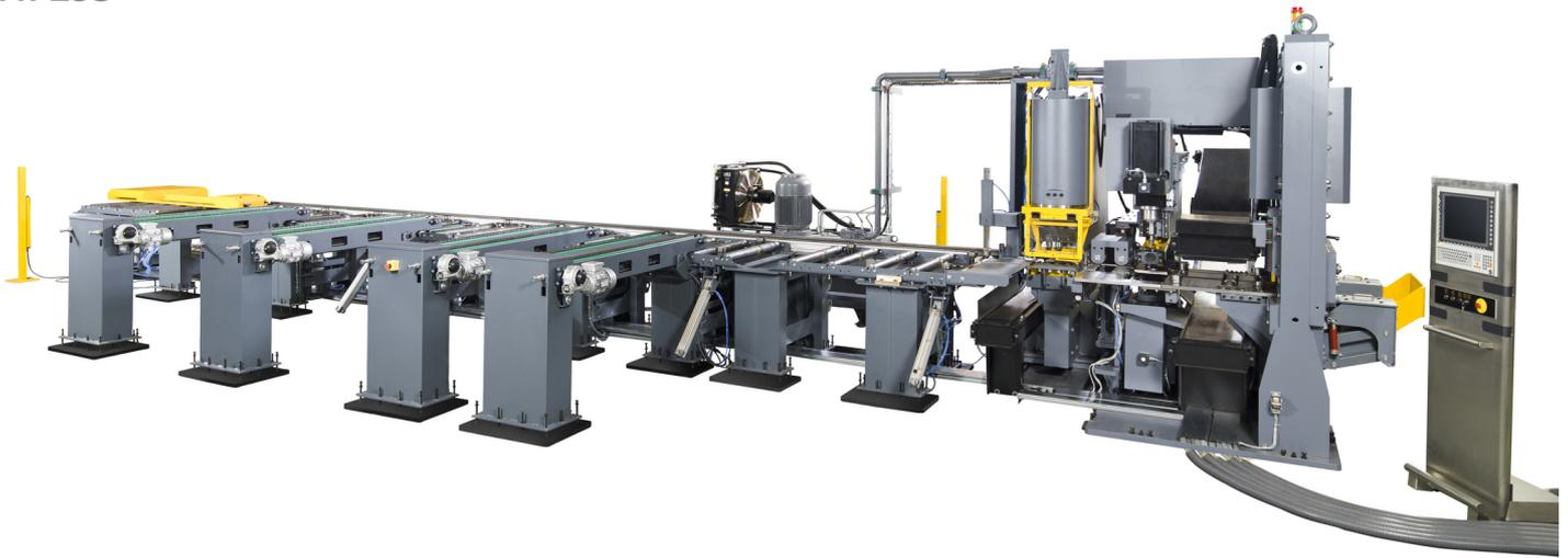
The ALFA PLUS not only includes the possibility of working with flat bars but also an angle bar. With this machine, a steel fabricator will be able to process both angles and flats to maximize their production output with all the same options as the smaller ALFA ranges. This machine will surpass the investment cost in no time with the additional options as the automatic infeed and outfeed.
