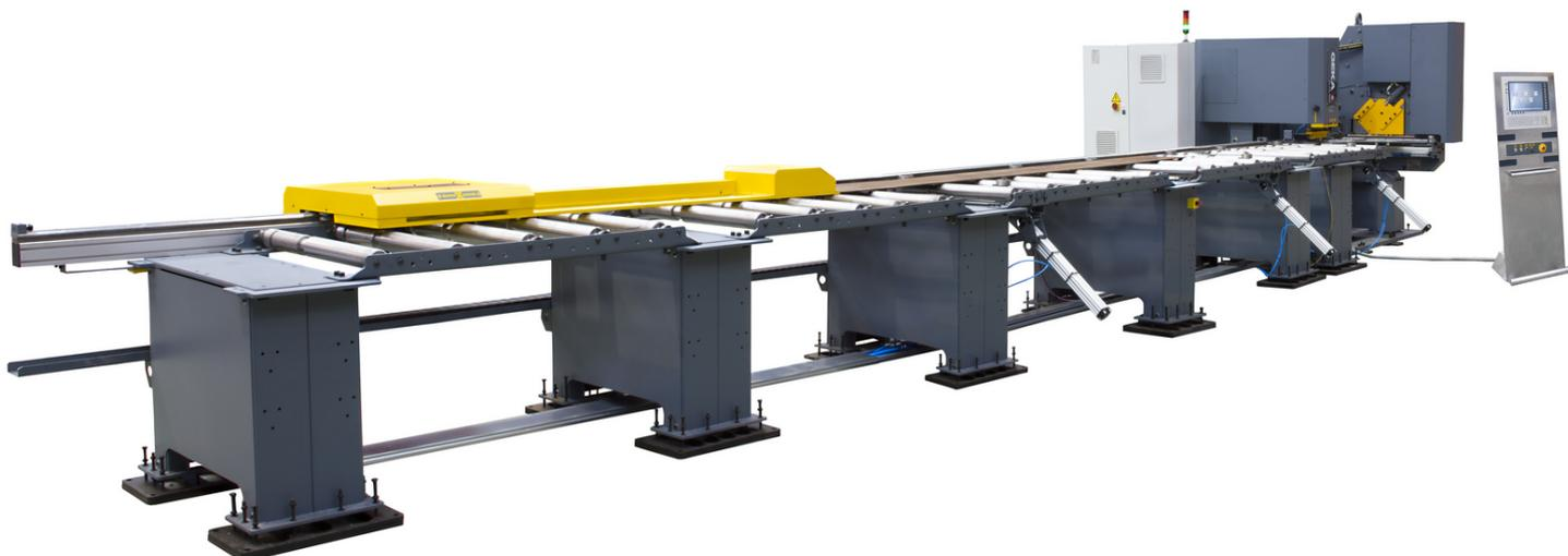
The ALFA series is a CNC punching and shearing machine specifically designed for steel fabricators that require medium and high output production. In the this ALFA version, the fabricator will be able to process flat bars from 6 to 12 meters and add a wide range of options like marking, drilling, mitre shearing and automatic loading and unloading to increase their production to a new level.
